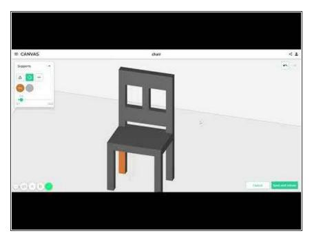
With the support tool on and using the facet or sphere tool, paint the model where you would like supports to be generated. Each painted region will generate supports vertically. With the tool off you may erase painted regions.
