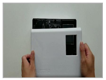
Turn Palette 2 off and remove the top lid by gently lifting from the sides.
