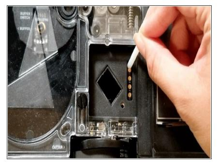
Check that the power supply and USB cable from your computer is plugged into Palette. Hold the white reset button down. You may use a thumbscrew or other tool if you prefer.
