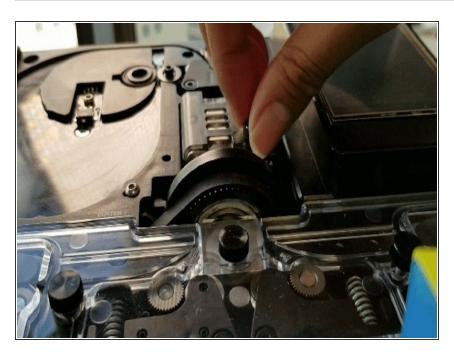
Remove the splice core by unscrewing the thumbscrew and lifting the splice core from the substructure.
