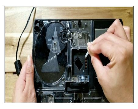
Hold the reset button, then turn the power switch on. Once Palette is on (you'll see the internal lights turn on),
