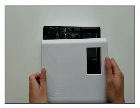
Turn Palette 2 off and remove the top lid by gently lifting from the sides.
