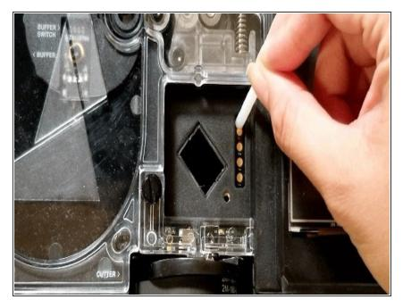
Check that the power supply and USB cable from your computer is plugged into Palette. Hold the white reset button down. You may use a thumbscrew or other tool if you prefer.
