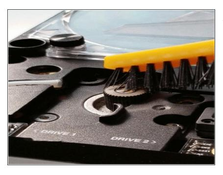
Clean the drive gears. We suggest using a wire brush to scrape the drive gears or to run tweezers along the groves, removing any residue or filament buildup. Compressed air will also help to clear any additional debris.
