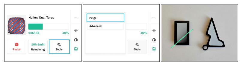
Monitoring calibration: To view calibration pings while a print is in progress, go to Tools > Pings from Palette's screen.
