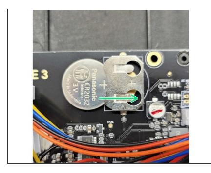
Remove the battery from the old main board, and insert into new main board. Insert the battery so that the (+) is on the right, and matches the position of the (+) symbol in its slot.
