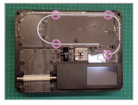
Remove the PTFE tube from fasteners and lift the collet before removing the entire buffer tube along with the brass retainer.
