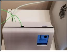
Load filament into the inputs, making sure not to use clear or transparent filament for any inputs as
