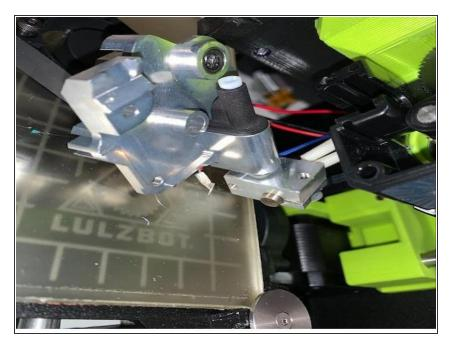
Allow to the extruder cool before reassembling.
