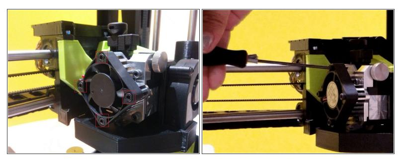
Turn off the printer. Remove 4 screws from the square fan. Gently pull the fan back and allow it to hang from the side. Place the 4 screws in a safe spot as they will be needed for reinstallation shortly.
