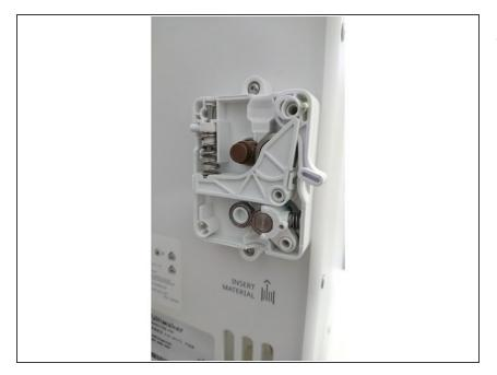
How to swap the extruder drive arm in the Ultimaker filament feeder on the back of the printer.
