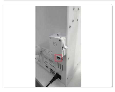
Install the Palette tube into the <u>extruder input</u>
