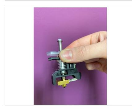
• How to install the short hot-end <u>PTFE sleeve into the hot-end.</u>
