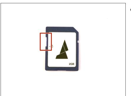
Please note the orientation of the SD card when inserting into Palette. When you're looking at Palette's screen, the Mosaic Logo should be facing you when inserting into your Palette. Please also check that the lock is off.
