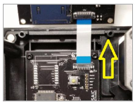
If you're still not able to read the files properly, we can check the connection of the SD card reader to the electronics tray as a last resort.
