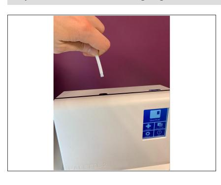
• Please disconnect the Palette 2 outgoing tube from Palette 2 by firmly pulling it out, this is a push fit connection so you will need to use a bit of force to remove it. Ensure that there is no filament in the path from this tube to the hotend. If there is, please remove the filament so that the path is clear.
