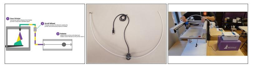
Positioning is really important! Positioning Palette or the Scroll Wheel incorrectly can result in weak splices and failed prints.
